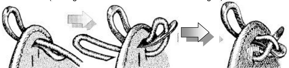
Use an awl to widen the holes and pass the loops through.
