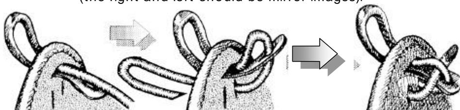
Use an awl to widen the holes and pass the loops through.
